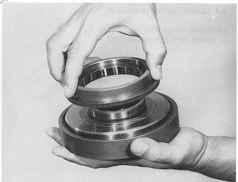
After removal of the snap ring disconnect freewheel inner ring from hollow gear.
