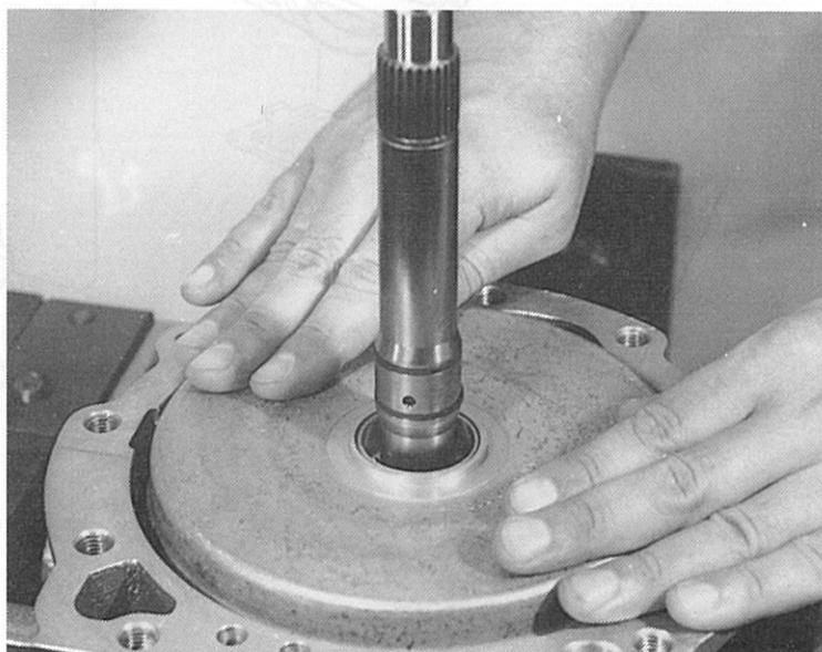
Insert thrust washer 02.060 and axle cage 02.050 into seat at cylinder A.
