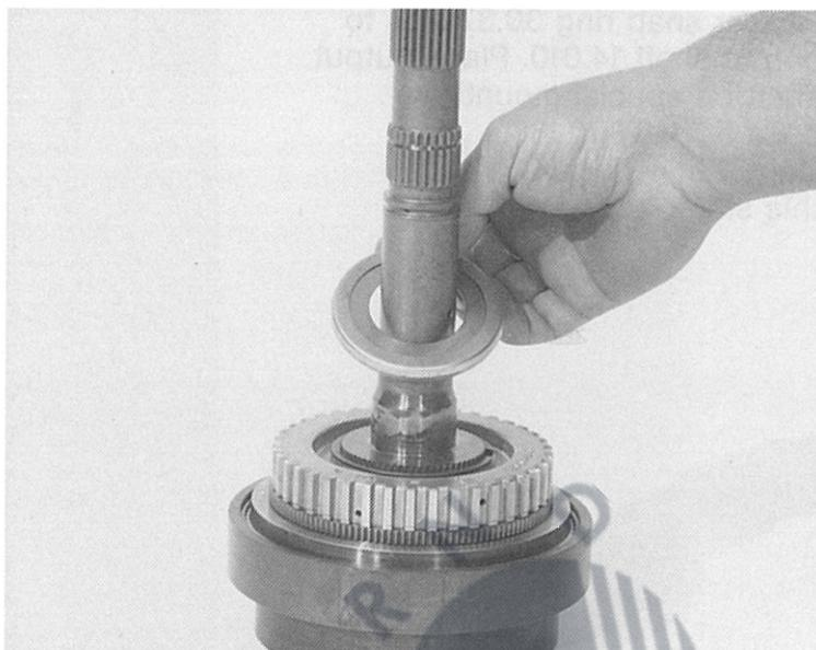
Install cylinder E assembly with turning motion.
