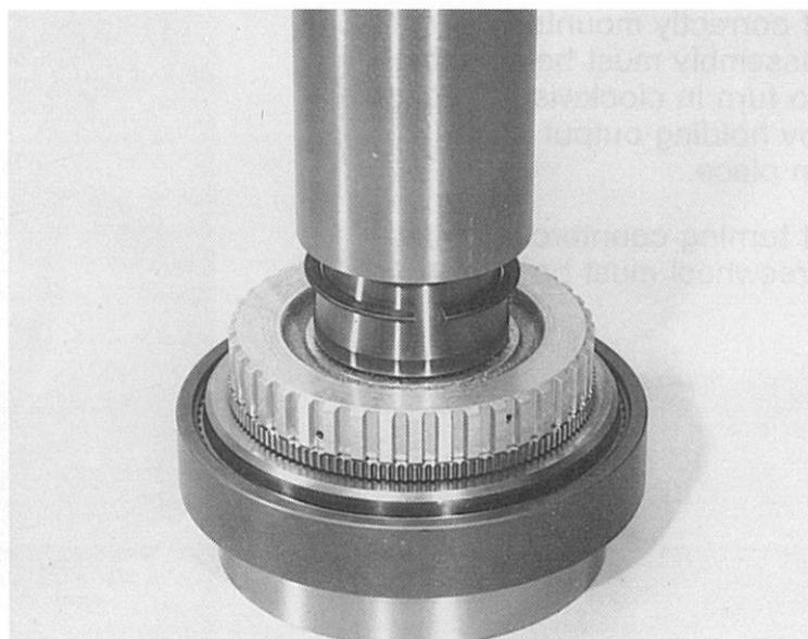
Install first steel thrust washer 30.142, second copper thrust washer 30.146 as shown in the picture.
