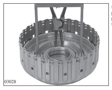
Using assembly hoop 5x46 909 247, press the cup spring down in the arbor press and remove the snap ring, using suitable pliers.
