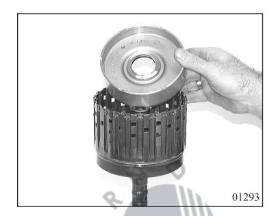
Put new O-ring seal 71.090 onto baffle plate 71.080. Insert cup spring 71.060 into cylinder E with the projections facing upwards and press in the baffle plate.
