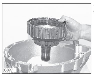
Insert complete clutch B into transmission housing.
