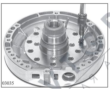
Unscrew the 11 countersunk-head machine screws (at the outer ring of the stator shaft) and remove them except for two on opposite sides. Strike the pump carefully with a plastic-faced hammer to drive it out on to these screws.
