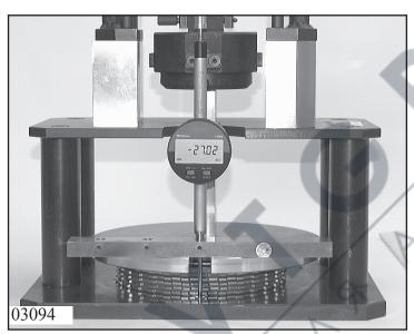
Determine thickness  $M_B$  of the clutch B disk cluster as described in Chapter 1.4.0 "Measuring the disk clusters".
