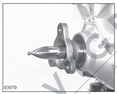
Place sealing ring 5x46 012 696 with press-in aid over drive shaft.
