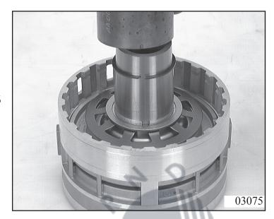
Turn cylinder CD by 180°. Put 2 O-ring seals 75.040 and 75.050 onto piston C 75.030 and press it into the cylinder.
