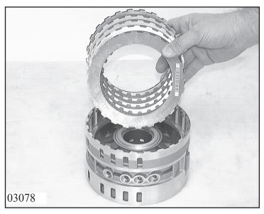
Insert complete clutch pack C into cylinder CD, starting with spring disk 75.100. Then insert an outer disk 75.140 and a lined disk 75.120 alternately. Secure the top outer disk 75.150 with snap ring 75.180. Clip needle bearing 73.300.
