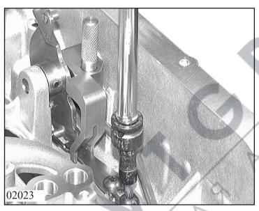
Detent spring with centering device Align 5x46 002 292 and in this position, tighten the detent spring. Tighten the screw on the output side first.
