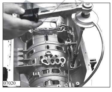
After this, use auxiliary tool 5w04 000 583 to turn farther by the amount of angular offset.
