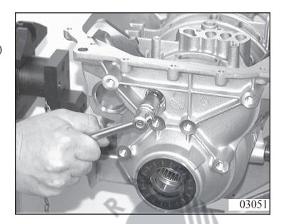
Press pin out of transmission casing. The ratchet with spring can then be taken off.
