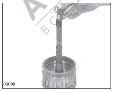
Put 3 new rectangular-section rings 71.190 and one o-ring 71.220 onto cylinder E 71.010 with input shaft.
