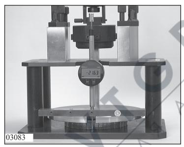
Determine thickness  $M_D$  of the brake D disc cluster as described in Chapter 1.4.0 "Measuring the disk clusters".
