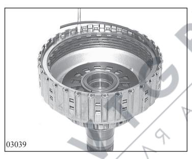
Next, turn the cylinder by 180 degrees, remove the snap ring at clutch B and take out the complete disk cluster.
