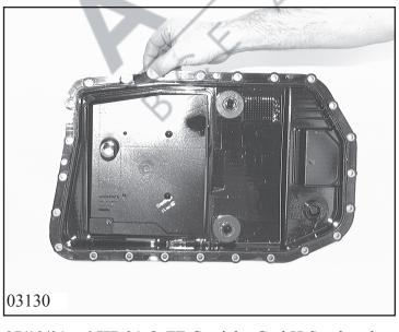
Put new O-ring seal 03.010/020 onto stub pipe of oil filter 03.010. Press new seal 03.010/014 into oil pan 03.010.
