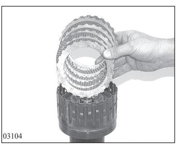
Insert complete clutch pack E. Start with spring disk 71.140, then insert outer disk 71.150 and lined disk 71.160 alternately. Insert final disk 71.170 and secure with snap ring 71.180.
