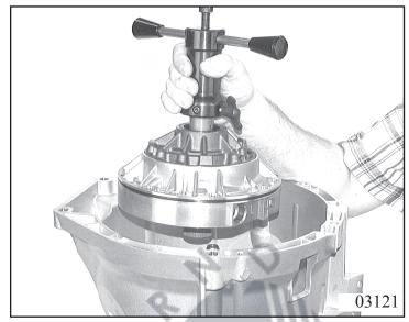
Tighten down the oil supply with 11 Torx screws 10.080 and new Usit rings as follows:
