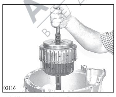
Align discs of clutch B, insert turret by hand and turn it in both directions until the discs engage fully in disc carrier B.
