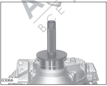
Press needle roller bearing 14.020 into transmission casing using mandrel 5x46 909 346 and supporting ring 5x46 909 347. Secure with snap ring 14.040
