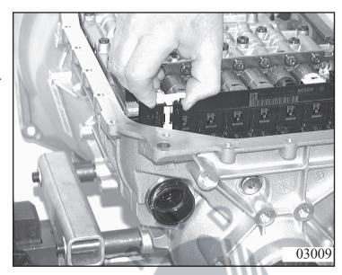
Unscrew and remove the **large-headed** screws (M6) and lift off the complete Mechatronic assembly.
