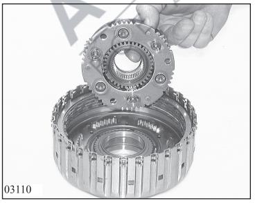
Insert sun wheel 32.010/210 with axial needle cage 32.010/190 facing the inside of the planet gear set 32.010.
