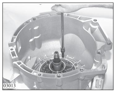
Turn the transmission by 90 degrees. Remove the complete oil supply system by unscrewing the 11 torx screws and taking them out complete with the Usit rings.
