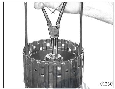
Plug one of the two oil feed holes and force piston E out with compressed air. Pull off the two O-ring seals.
