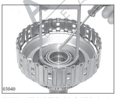
Using assembly hoop 5x46 909 248, press cup spring B out in the arbor press. Remove the split retaining ring and take out the divided cup spring.
