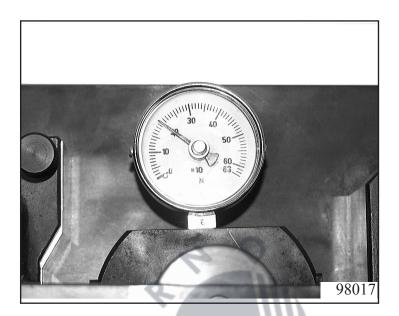
Next, place measuring bar 5p01 000 330 on the measuring plate, place the measuring foot of the dial gauge in the groove of the measuring plate on the upper disk of the disk cluster, and set the dial gauge to "0".
