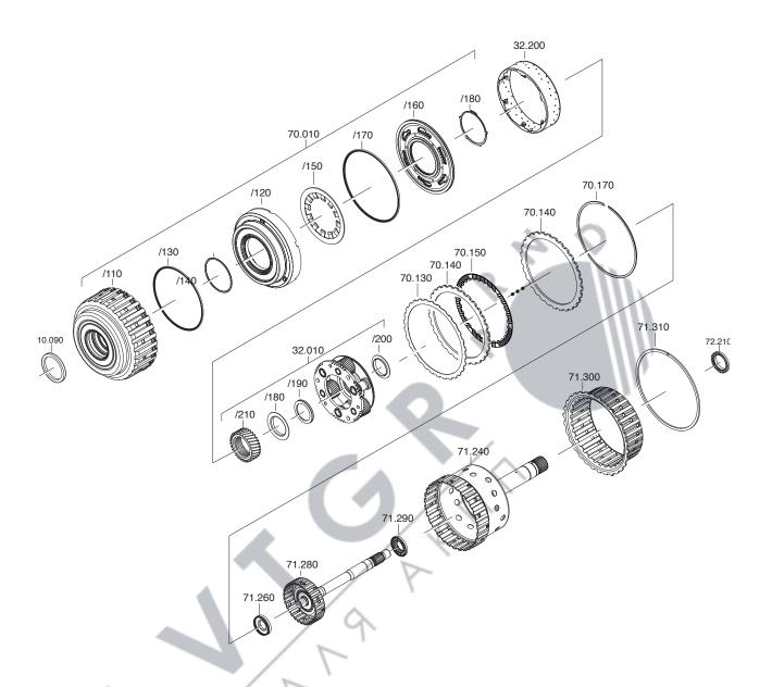
Put 1 new prof. seal ring 70.010/130 and 1 new O-ring seal 70.010/140 onto piston A 70.010/120.
