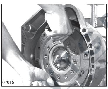
Remove the converter holding bracket and take out the converter, holding it by the two converter puller handles 5x56 000 090.
