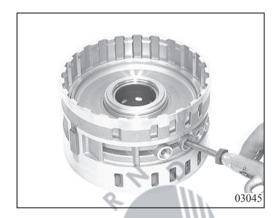
Apply compressed air carefully to the oil feed hole and force out piston D. Pull off 1 O-ring seal from cylinder D and 3 O-ring seals from the piston.
