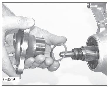
Place reversing disk 14.130 over drive shaft, push flange onto output shaft.
