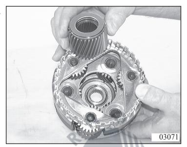
Turn transmission with converter bell upwards.
