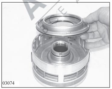
Drive 2 shaft keys 75.010/030, /040 in centrally at cylinder CD 75.010, using a plastic hammer.
