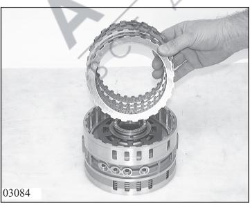
Insert complete clutch pack D into cylinder CD, starting with spring clutch disk 73.150 and then insert lined disk 73.170 and outer disk 73.160 alternately. Secure the last outer disk 73.180 with snap ring 73.190.
