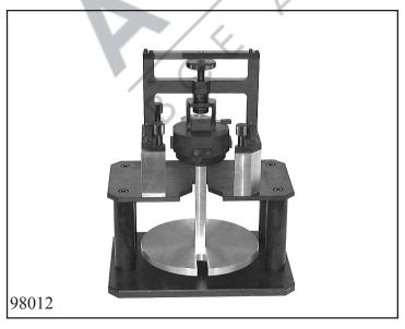
Tighten the 4 knurled screws 5p01 000 329 to secure the adjusting fixture firmly with the height measuring fixtures by way of the spacers.
