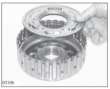
Insert cup spring 70.010/150. Put prof. seal ring 70.010/170 onto baffle plate 70.010/160 and insert the baffle plate into the cylinder.
