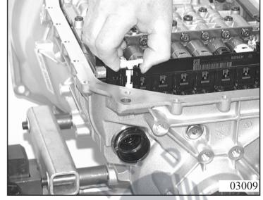
Unscrew and remove the **large-headed** screws (M6) and lift off the complete Mechatronic assembly.
