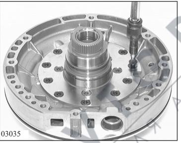
Unscrew the 11 countersunk-head machine screws (at the outer ring of the stator shaft) and remove them except for two on opposite sides. Strike the pump carefully with a plastic-faced hammer to drive it out on to these screws.
