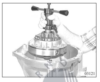
Tighten down the oil supply with 11 Torx screws 10.080 and new Usit rings as follows:
