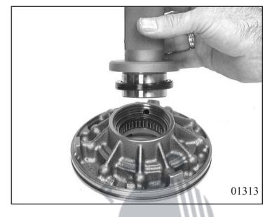
Put on new O-ring seal 10.020. Lubricate the pump wheel and internal ring gear slightly before assembly. Then assemble the pump in such a way that one marking is visible on the pump wheel and the internal ring gear each.
