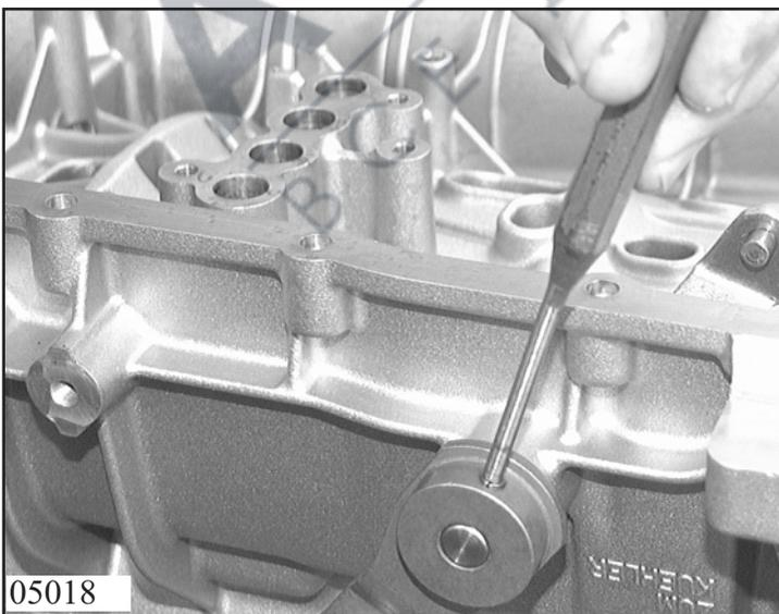
Remove clamping sleeve from notched disc. Withdraw selection shaft. Remove detent disc with connecting rod.
