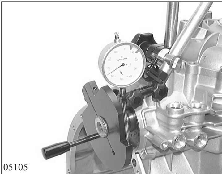
Lock the flank clearance measuring disc 5x46 010 384 on the lateral shaft.
