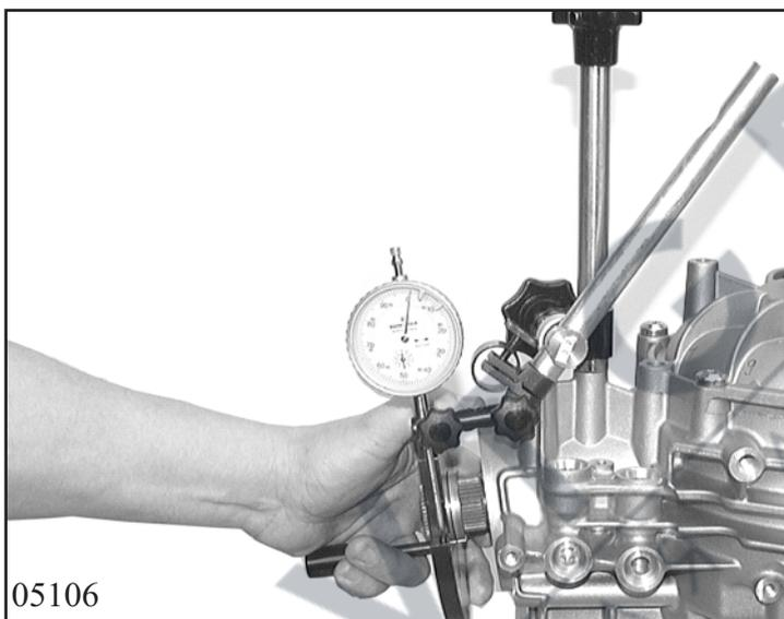
Turn the pinion shaft to one side to the pinion/bevel gear teeth stop. Set the dial to "0".
