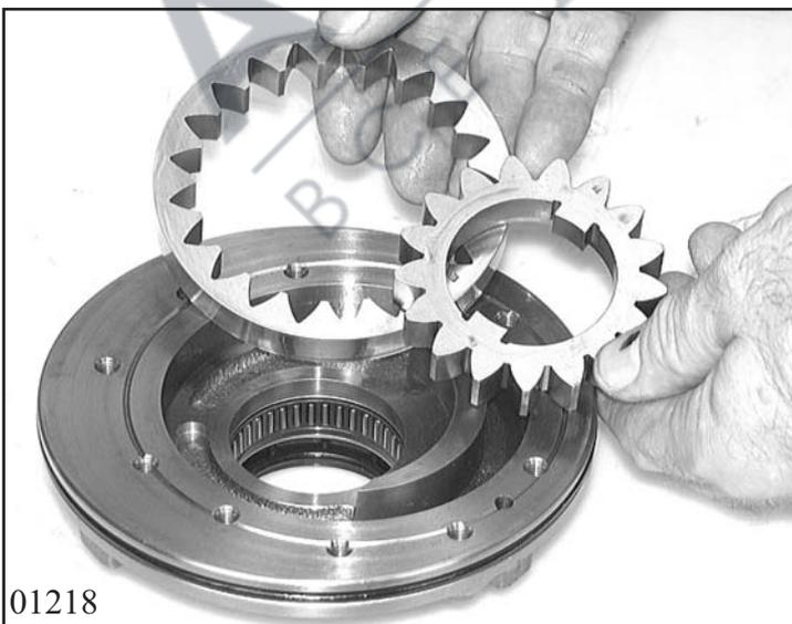
Remove O-ring type sealing ring. The pump can be disassembled by removing the pump wheel and the internal geared wheel.
