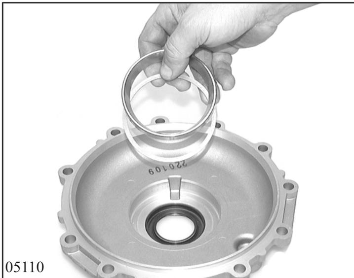
Determine the disc's overall thickness  $M_G$  by measuring the adjustment spacer thickness 35.080 and 35.110.  $\Rightarrow M_U, M_O$
