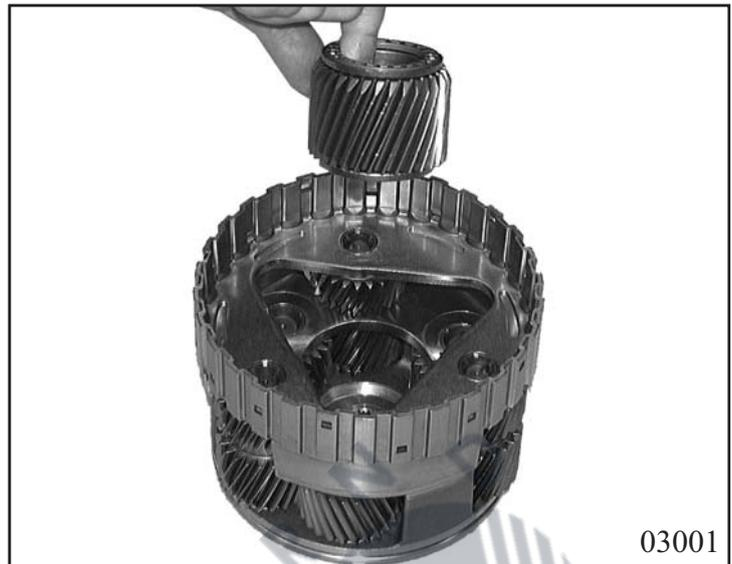
Rotate gearbox with converter bell side upwards. Clip bearing 42.210 in planetary gear set 42.010. Insert disc 42.200 and planetary gear set in gearbox housing.
