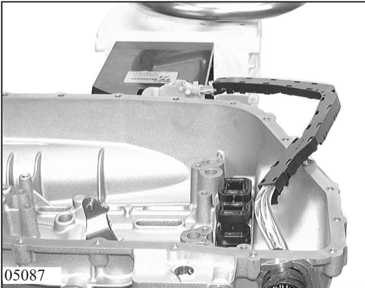
Pull on 2 new O-ring type sealing rings onto cable plugs. Plug in the plugs of the wiring harness into the gearbox housing and fix with locking plate 27.530. Then put Mechatronic on, press connectors into Mechatronic and clip cable guide onto screw heads.
