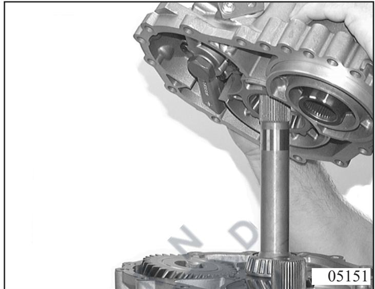
Insert output wheel 38.100 in intermediate housing. Fix intermediate housing to gearbox housing with 19 torx screws 38.550.
