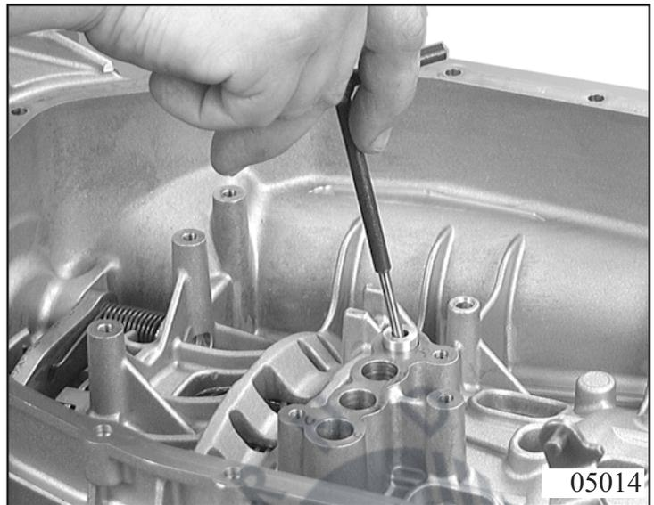
With puller handle 5x95 000 410 pull out the 4 sealing sleeves sitting on the bottom of the bore.
