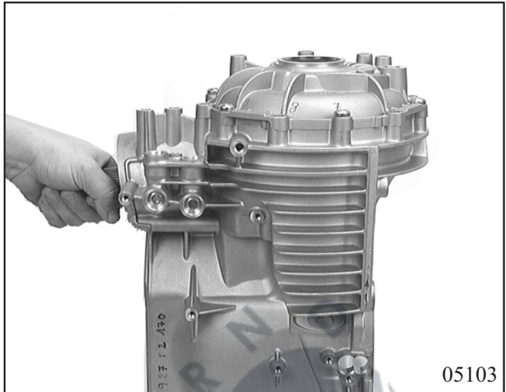
Screw in the measuring tripod's standing column with M10 in the compatible gearbox housing thread. Lock the transverse holder so that the dial sensor is aligned to the measuring plate centrally and in a right angle. Set the dial to "0".
