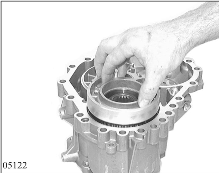
Insert drive wheel 38.030 in intermediate housing. Put on bearing ring 38.070 and fix with screw 38.080
