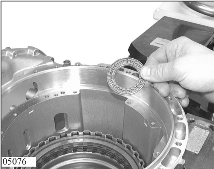
Present axial needle cage 72.210 to the hub of cylinder B. For installation position of the bearing, see picture.
