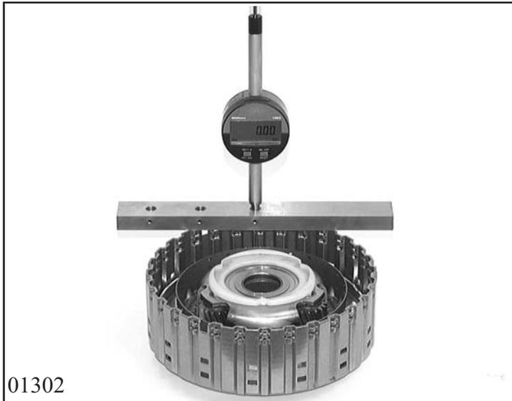
Measure the clutch A installation space  $E_A$  with measuring bar 5p01 000 330. To do this, place the measuring bar 5p01 000 330 on the edge of clutch A's cylinder. Place the measuring base on the highest area of the disc support surface at the piston and set dial to "0". Pull the measuring sensor upwards, insert it into the snap ring groove and press against the upper groove edge.
