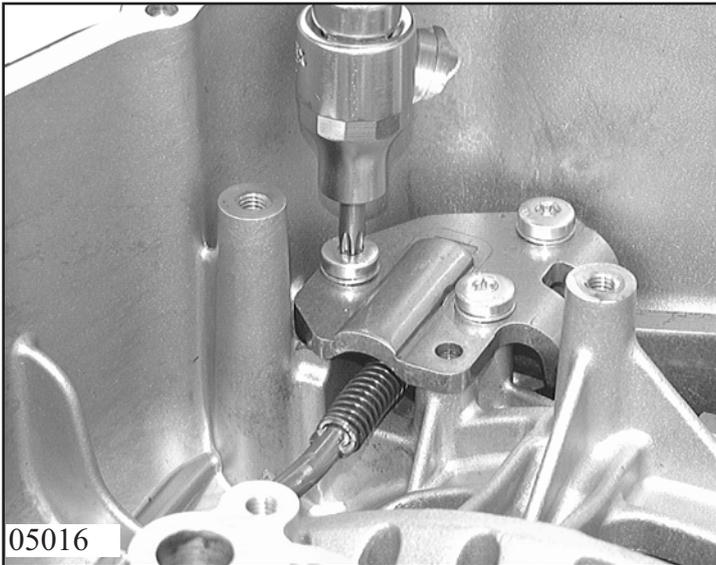
Press out parking lock pins to the rear. Remove pawl with spring.
