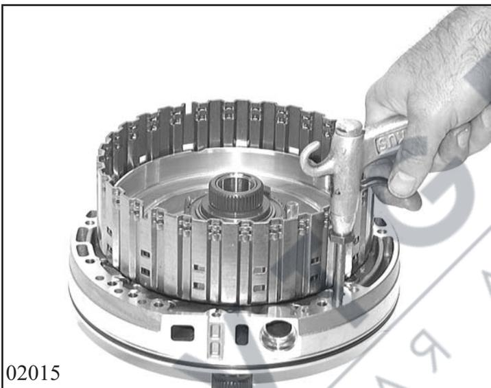
Put cylinder A on oil supply and press out the piston with compressed air. Remove 2 O-ring type sealing rings from piston A. Remove cylinder A from oil supply.
