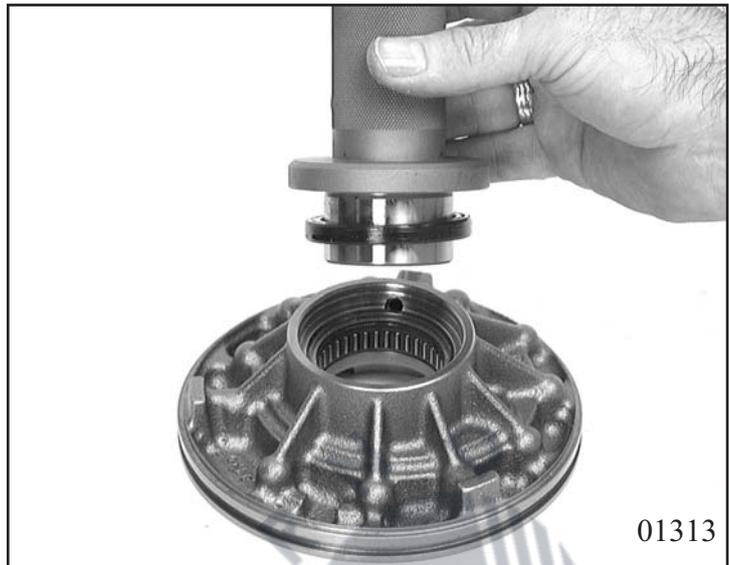
Pull on new O-ring type sealing ring 10.020. Slightly lubricate pump impeller and internal geared wheel with oil before assembly. Then assemble pump in such a way that markings are visible at each of the pump impeller and internal geared wheel.
