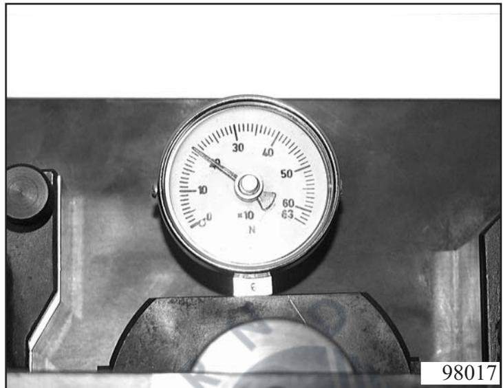
Then place the measuring bar 5p01 000 330 on the measuring plate. Lay the measuring base of the dial gauge in the measuring plate groove onto the disc set's uppermost disc and set dial to "0".
