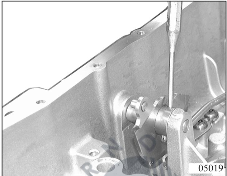
Remove shaft sealing ring with suitable tool.
