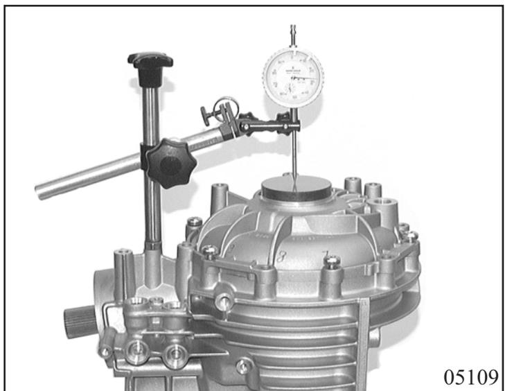
According to the test instruction 1068 700 067, the measured value  $M_D$  must be between  $M_{Dmin} = 0.18\text{mm}$  and  $M_{Dmax} = 0.28\text{ mm preload}$ .
