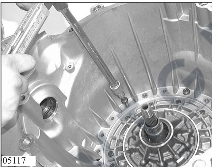
Mount converter bell on gearbox housing and fix with 18 screws 22.300.
