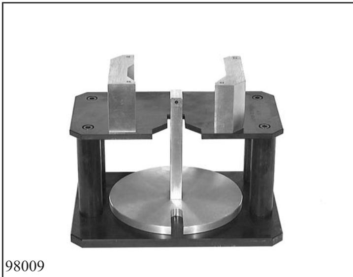
Turn the adjustment device 5p01 001 458 to the upper stop position with the knurled screw. Hang the force measuring unit 5p01 000 329 into the adjustment device.
