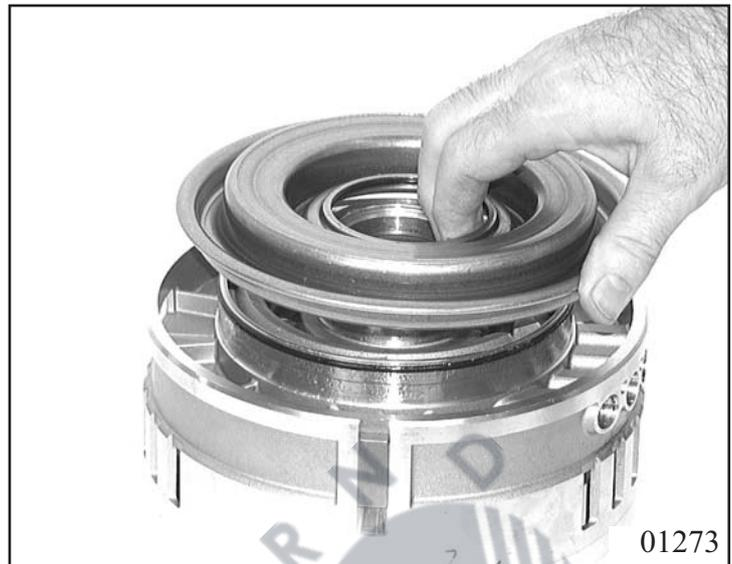
Pull on 1 round sealing ring 73.070 onto baffle D 73.060 and press this into piston D.
