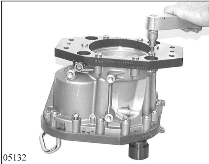
Turn the housing by 180° and stabilise with appropriate little blocks. Screw the plate 5p01 003 114 onto the intermediate housing sealing area with 7 screws.
