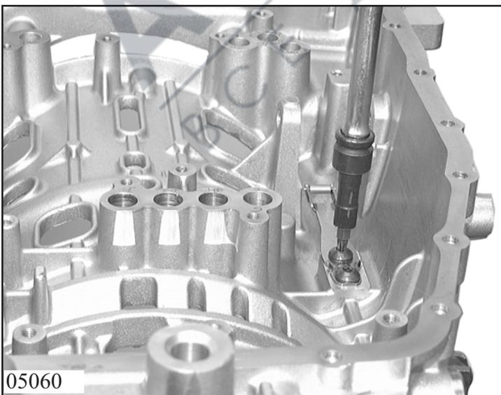
Tighten detent spring 06.094 with 2 Torx screws 06.100.
