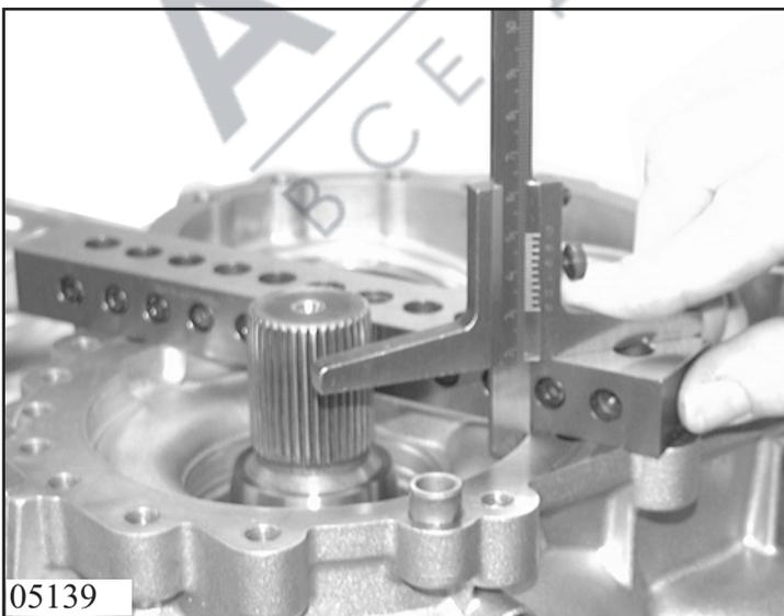
Place the depth gauge on the intermediate housing/gearbox housing sealing surface and measure down 3 times offset by  $120^\circ$  to the input shaft bearing seat. Calculate the average of the measured values. Calculate the average of the measured values  $M_1, M_2, M_3 \Rightarrow M_{RA}$
