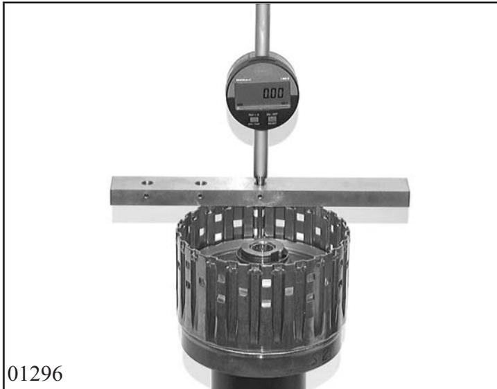
Measure the clutch E installation space  $E_E$  with measuring bar 5p01 000 330. To do this, place the measuring bar 5p01 000 330 on the edge of clutch E's cylinder. Place the measuring base on the highest area of the disc support surface at the piston and set dial to "0". Pull the measuring sensor upwards, insert it into the snap ring groove and press against the upper groove edge.
