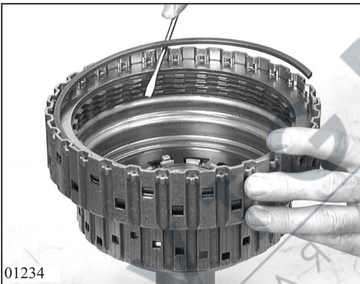
Now rotate cylinder by 180° and release the snap ring of clutch B and remove the complete disc set.
