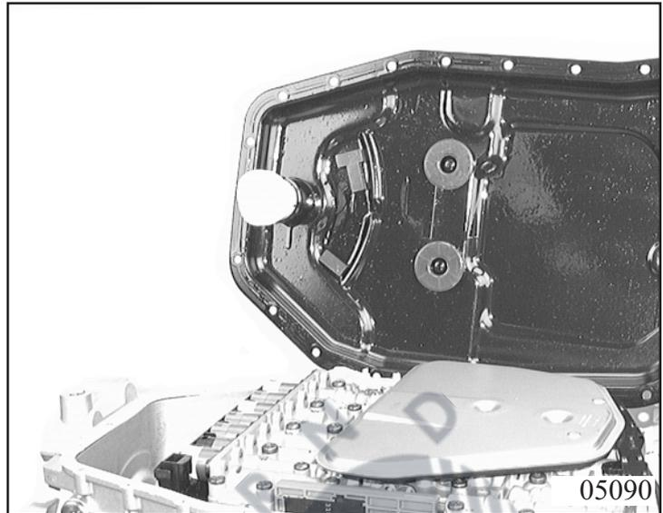
Screw in oil outlet 03.010/120 and filler screw 03.010/130 into oil pan. Screw in filler screw of differential 35.350 into differential housing.
