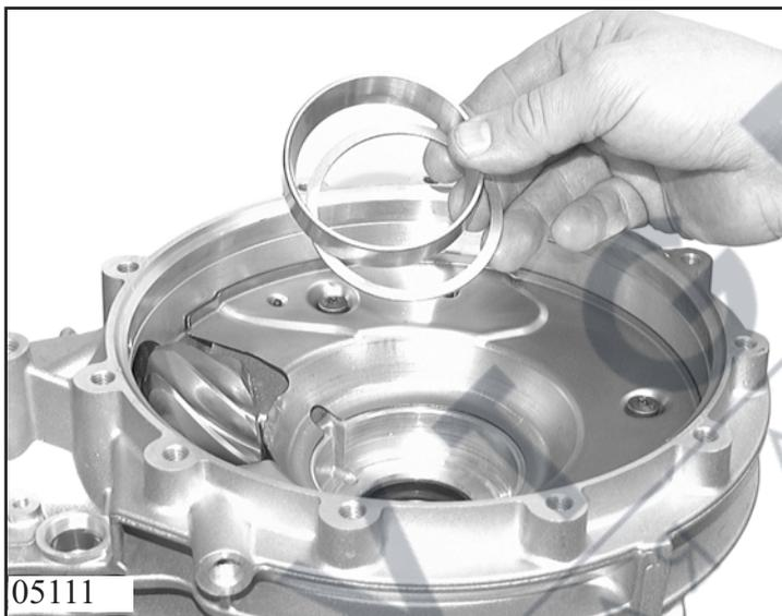
Insert the removed adjustment spacer 35.080 with the bearing ring 35.010/120 in the differential housing. This can usually be done by hand. The bearing seat may have to be heated slightly with a hot-air blower.
