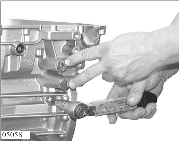
Screw in 2 new oil cooler screws into gearbox housing.
