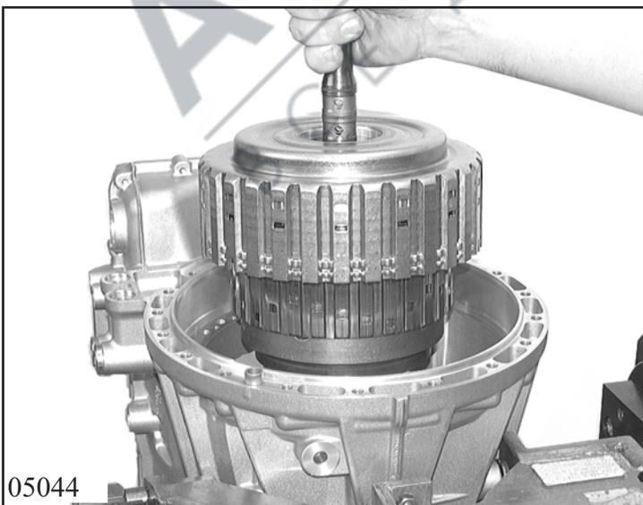
Take out spacer. Lift out tower (drive with clutches A and E) by hand. Insert tower in holding device 5x46 000 917 and remove device.
