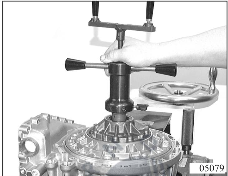
Screw in oil system with 14 Torx screws with new Usit rings as follows:
