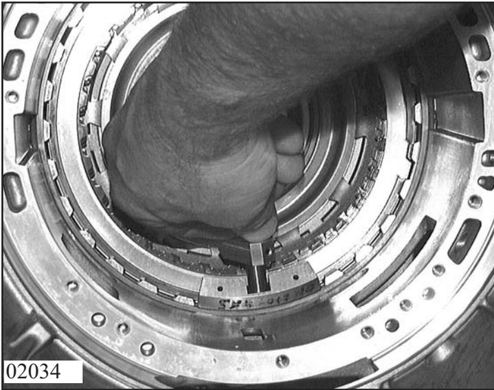
Secure in gearbox housing with snap ring 73.210 .
