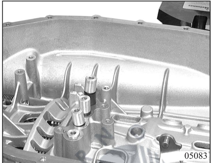
Insert adapter 27.460 in gearbox housing.
