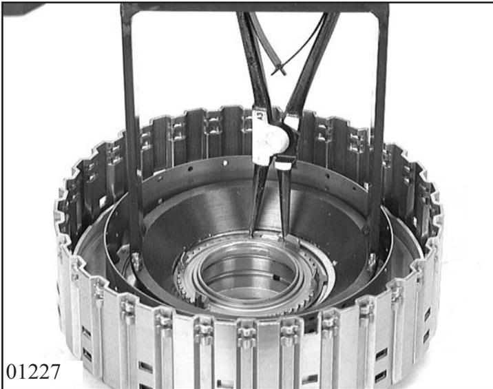
Press out the cup spring downwards under the mandrel press with assembly bracket 5x46 002 566 ,remove snap ring with suitable pliers. Remove planetary carrier and diaphragm spring. Take off O-ring type sealing ring from planetary carrier.
