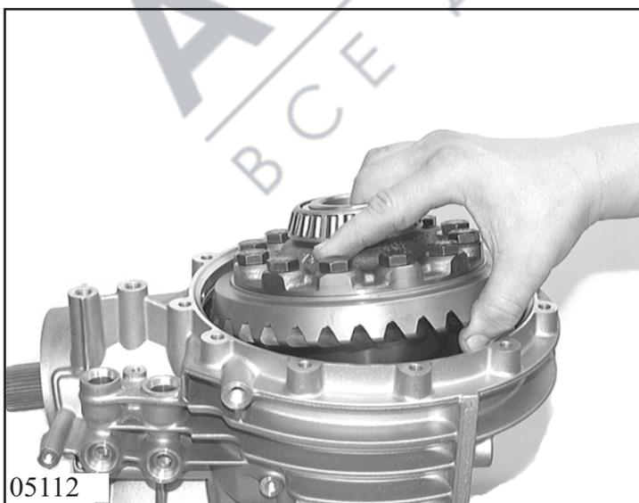
Insert the differential in the gearbox housing. Put on the differential cover.
