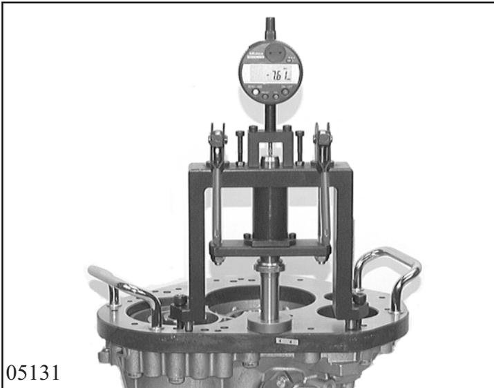
Place the pressure stamp 5p01 033 115 on the plate and set the dial from the stirrup to the fixed value  $M_{FA}$  (= -7.61) engraved on the measuring stirrup.
