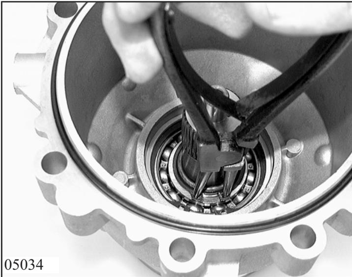
Lever out shaft sealing ring. Remove snap ring using pliers. Press out ball bearings under a mandrel press.
