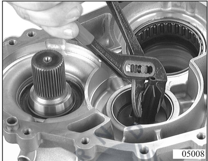
Remove outer bearing race tool with 5x46 021 007 and basic unit 5x46 022 002. Remove setting shim.
