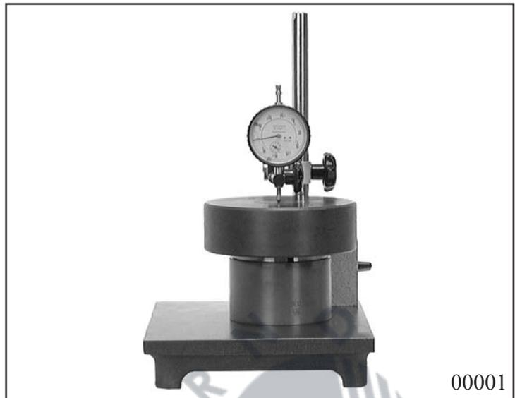
Place the differential side of the bearing inner ring on the measuring plate.
