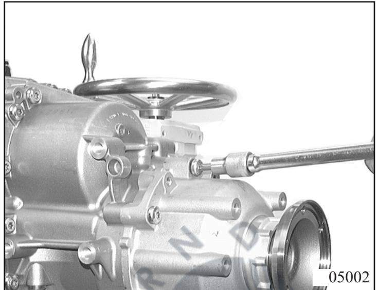
Take out bearing ring with setting shim. Loosen 19 screws, release intermediate housing from gearbox housing with plastic hammer and allow oil to drain off. Rotate gearbox by 90°.
