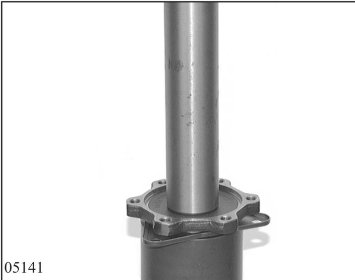
Press in flanged shaft 35.260/110 into the bearing 35.260/130 through the cover 35.260/120 under the mandrel press. Secure with half-moon ring 35.260/140. Use a suitable assembly tool for this.
