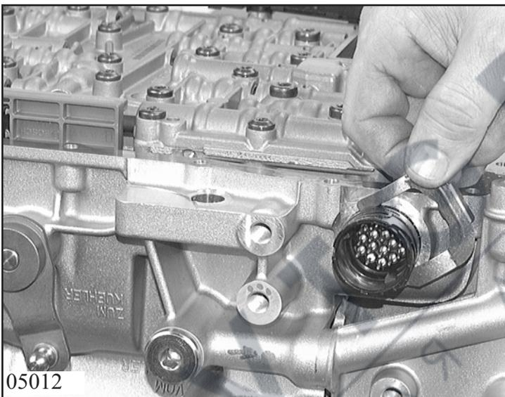
Loosen 11 large head screws and remove the Mechatronic. Take off adapters. Remove wiring harness from Mechatronic.
