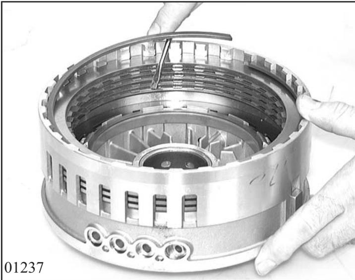
Release brake C snap ring and remove complete disc set.
