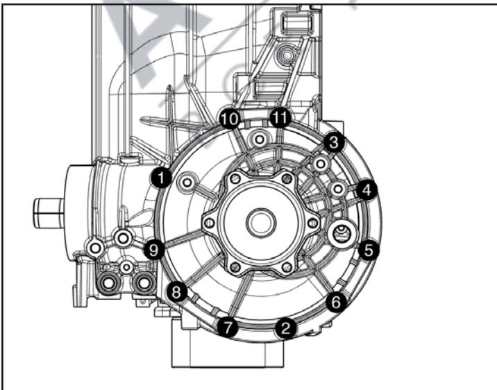
Tighten the differential cover torques according to the numbering:
