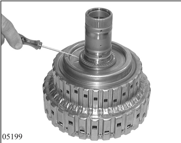
Unclip needle bearing from clutch B carrier.
