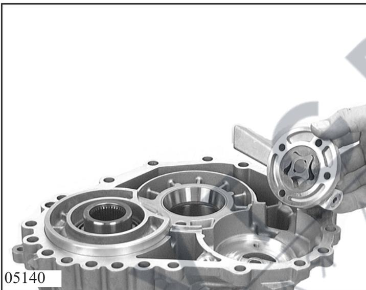
Insert pump internal geared wheel 38.300 in pump 38.300 and bolt pump in intermediate housing with 4 screws 38.390.
