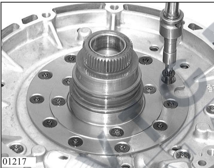
Loosen 11 off hexagon headscrews (countersunk head – outer ring idler wheel shaft), partially unscrew 2 off opposing cheese head screws. Drive out pump by carefully striking these screws with the plastic hammer.
