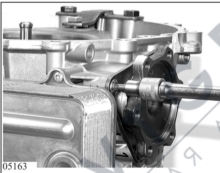
Rotate gearbox with converter upwards. Insert flanged shaft through converter bell into differential. Fasten cover with 3 screws 35.430.
