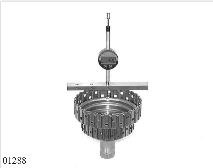
Measure the clutch B installation space  $E_B$  with measuring bar 5p01 000 330. To do this, place the measuring bar 5p01 000 330 on the edge of clutch B's cylinder. Place the measuring base on the highest area of the disc support surface at the piston and set dial to "0". Pull the measuring sensor upwards, insert it into the snap ring groove and press against the upper groove edge.
