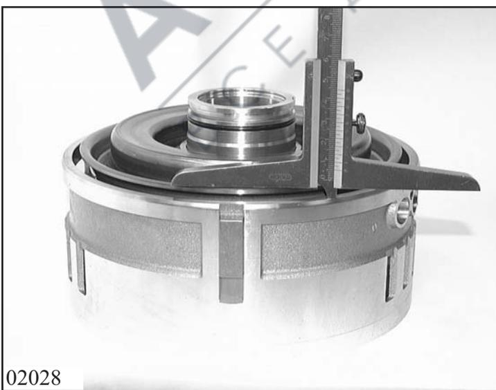
Measure down from the piston to the CD cylinder support surface and read the measured value. ⇨  $M_{DB}$
