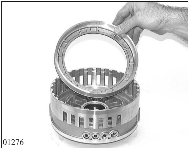
Rotate cylinder CD by 180°. Pull on 2 round sealing rings 75.040 and 75.050 onto piston C 75.030 and press these into the cylinder.
