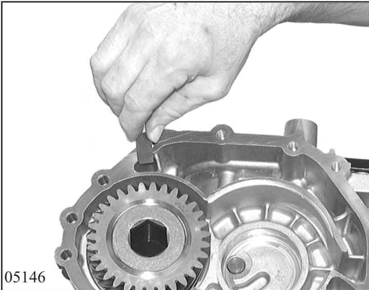
Heat up seat of bearing shell to approx. 70°C with hot-air blower. Press in new oil dispenser 37.010 into seat of front axle shaft. Insert setting shims for front axle shaft 37.050 and drive wheel 38.050 as well as bearing shells 38.020/150 in gearbox housing.
