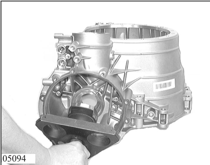
Turn the converter bell by 90° (converter bell downwards).
