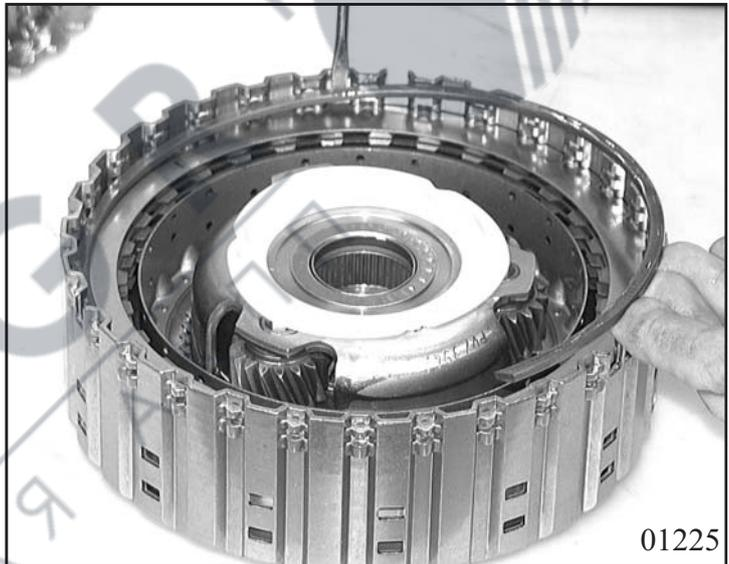
Lever out snap ring from planetary carrier and remove planetary carrier from cylinder A. Carefully unclip oil catch bowl. Remove snap ring and sun wheel from planetary carrier and lever out axial needle cage.
