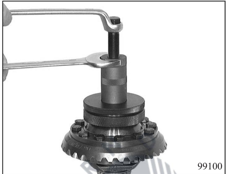
Loosen 12 screws of the crown wheel with device 5x46 002167 clamped in vice and separate crown wheel, possibly with plastic mandrel. Take differential out of device, rotate by 180° and push pins out.
