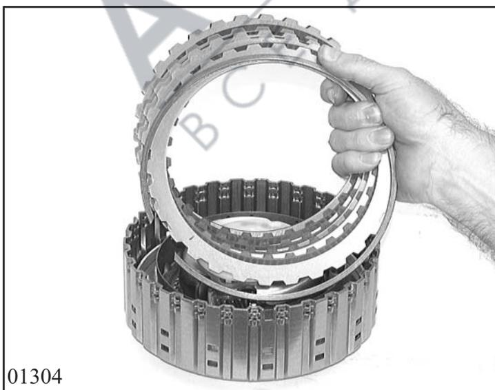
Insert complete disc set A. Starting with spring disc 70.130, then alternately insert outer disc 70.140 and lining disc 70.150.
