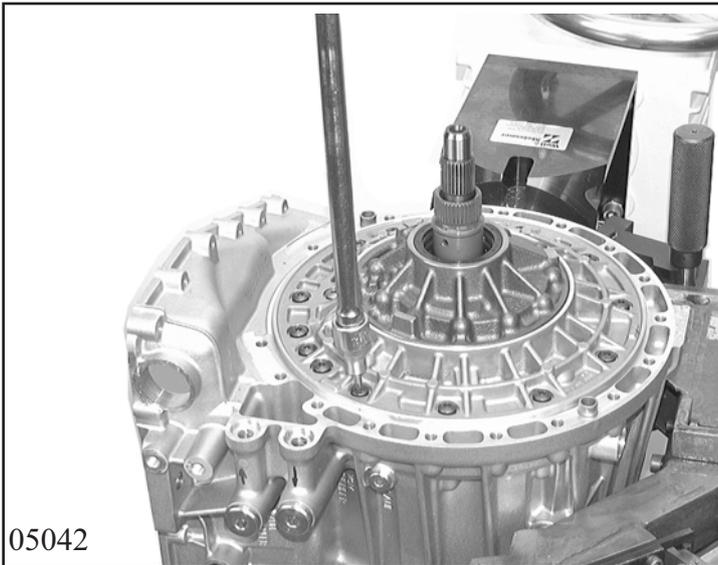
Remove complete oil system. In addition loosen 14 Torx screws and remove with the usit rings.
