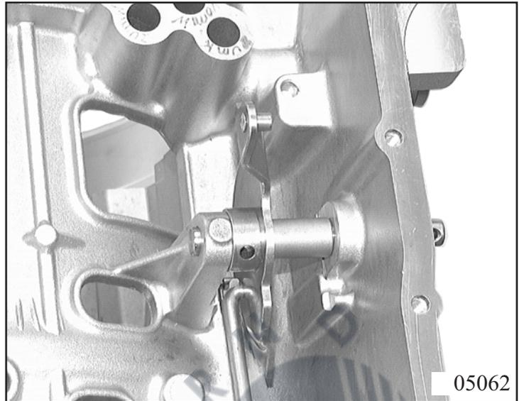
Drive in new locking pin 06.060 into position with driving in bolt 5x46 000 291 or a suitable mandrel.
