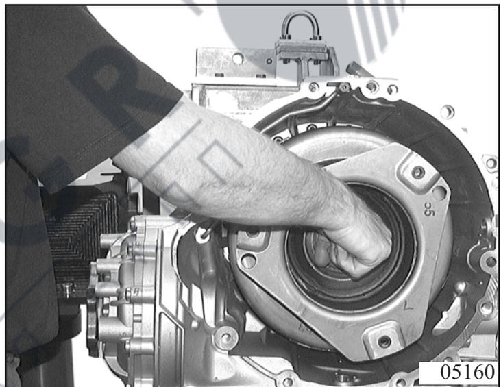
Screw on converter retainer 97.010 with 1 screw 97.020 and screw. 97.030.
