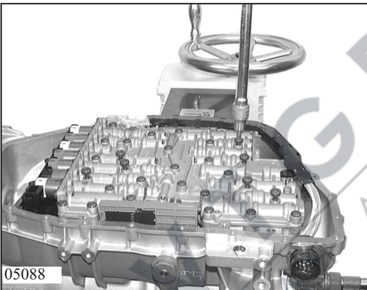
Suspend parking and/or latching disc in the groove of the piston rod. Align Mechatronic, press in by hand and fasten with 7 cylinder screws 27.450, as well as 4 cylinder screws 27.500. Engage the plugs of the wiring harness in the Mechatronic and press in the cable guide clips.
