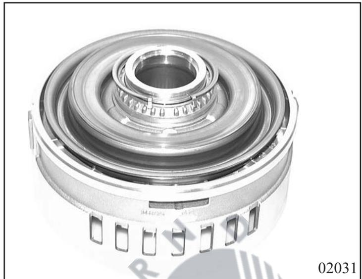
Carefully press out piston D via the oil supply bore with compressed air. Keep the two other bores closed during this. Remove 2 O-ring type sealing rings from cylinder D and 1 O-ring type sealing ring from the piston.
