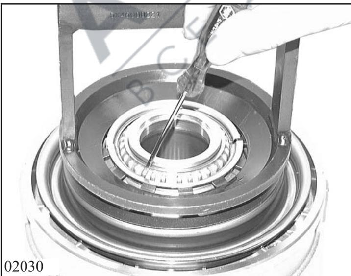
Rotate cylinder and press down cup spring D with 5x46 000 221 assembly bracket under the mandrel press, withdraw divided guard ring and remove cup spring.
