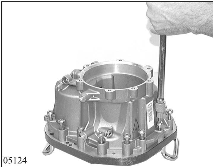
Insert the input gear in the intermediate housing.
