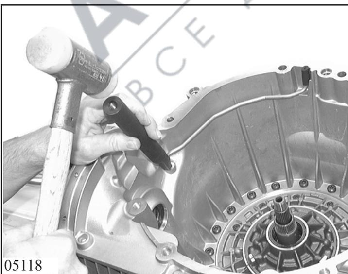
Pull O-ring type sealing ring 22.074 onto breather 22.070 and drive in with impact tool 5x46 001 525 or 5x46 001 411. If necessary, drive in 2 new guide bushes 01.110.
