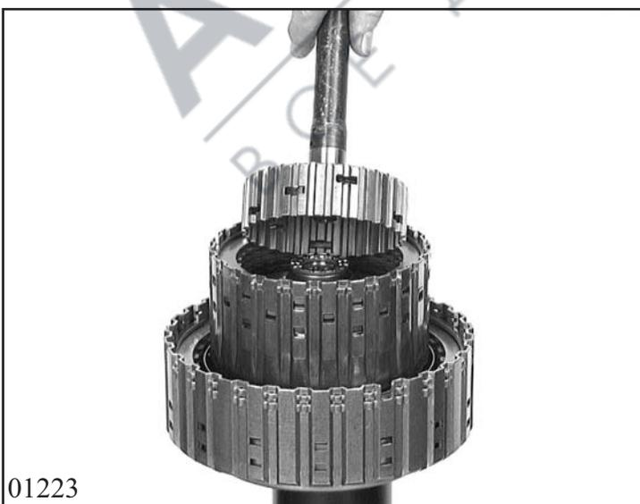
Lift off intermediate shaft with inner disc carrier E. Lever out axial needle bearing.
