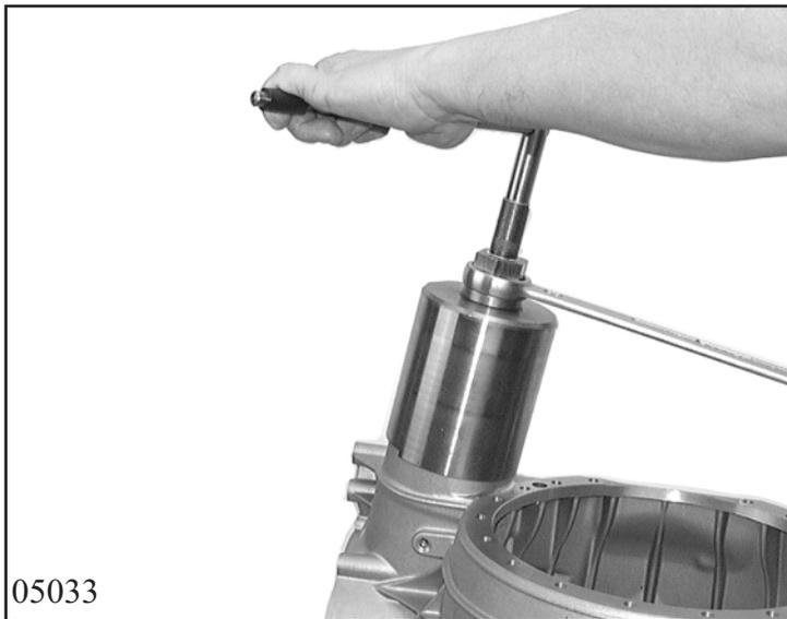
Withdraw pinion shaft from converter bell with tool 5x46 909 305. Press out shaft sealing ring of the flanged shaft from the converter bell.
