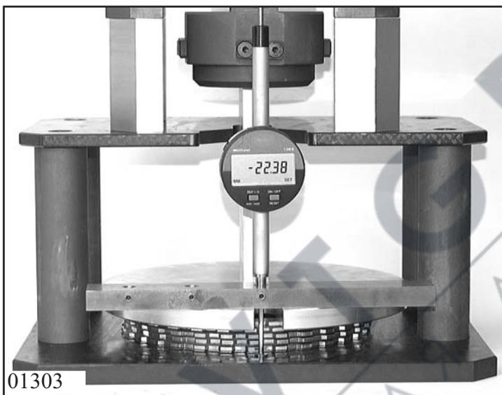
Measure the thickness  $M_A$  of clutch A's disc set as described in **Chapter 1.4.0 Measuring the Disc Sets**.
