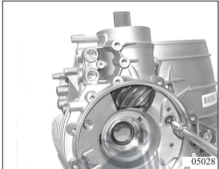
Remove external bearing cup with setting shim from converter bell.
