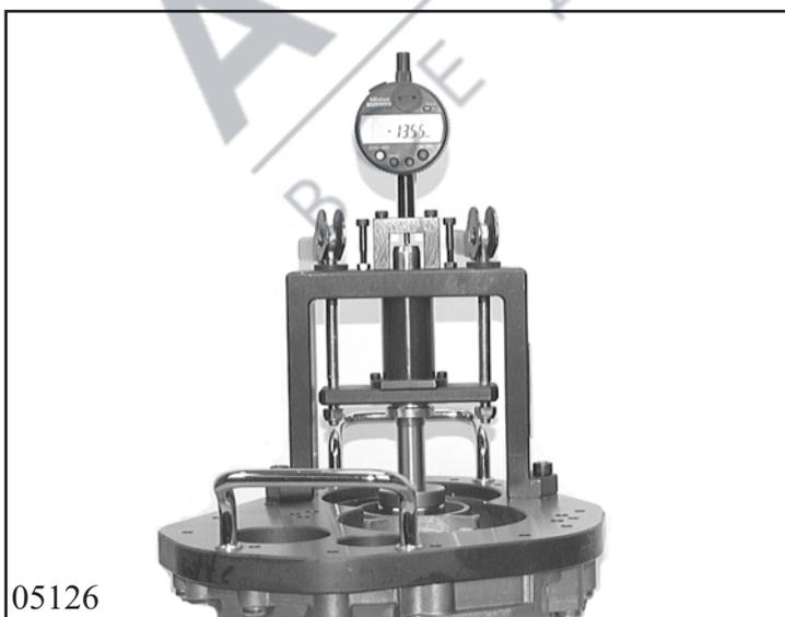
Place the stamp and stirrup on the input wheel and bolt on.
