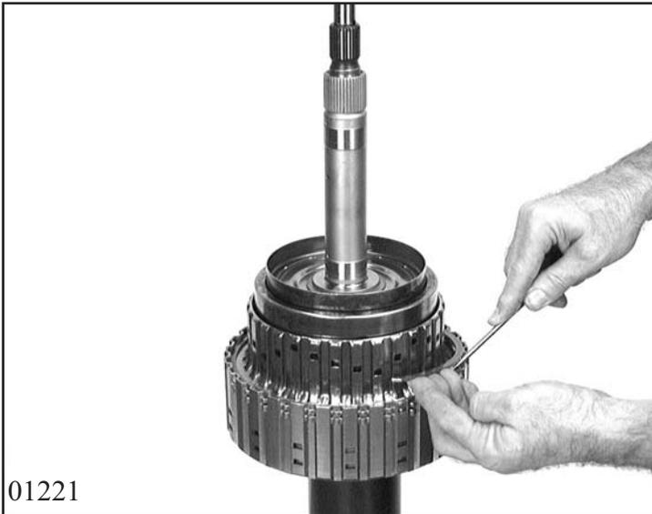
Place tower with drive shaft in device 5x46 000 917.
