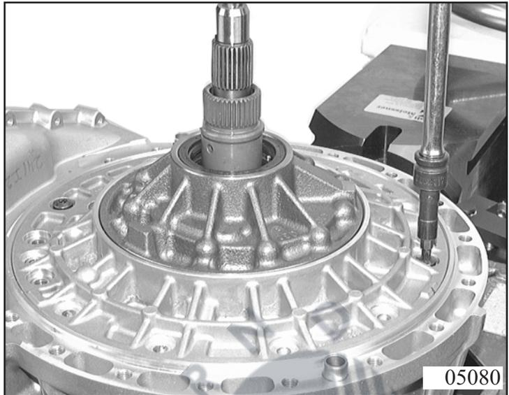
Put the measuring device 5p01 002 379 over the drive shaft teeth and lock about 2 mm above the stator shaft with the set screw.
