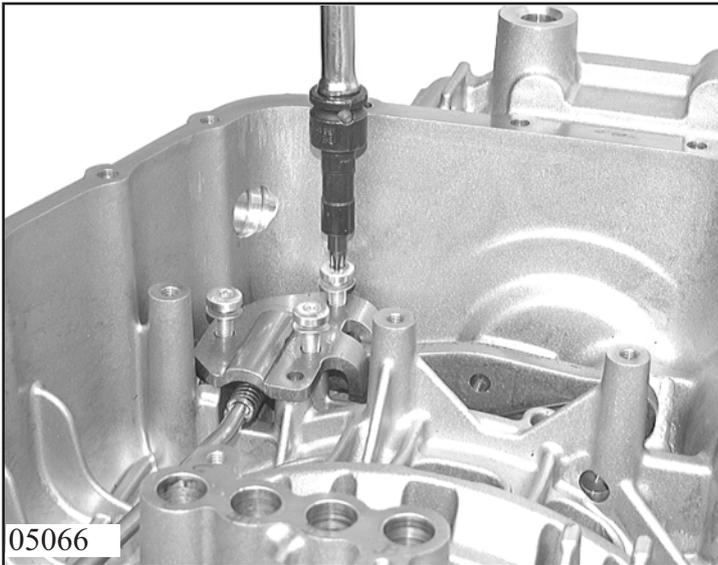
Press down pawl, and fasten guide plate 24.110 with 3 Torx screws 24.120 .
