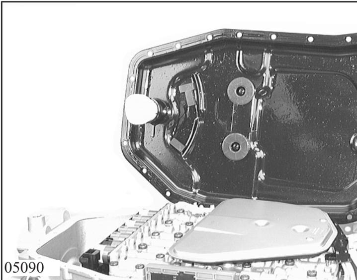
Remove locking plate from the wiring harness plug.
