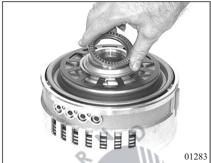
Insert complete disc set D into housing, starting with end disc 73.260 and then alternating lining disc 73.250 and outer disc 73.240 . Finish with spring disc 73.230.
