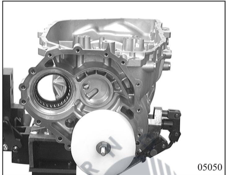
Press shaft sealing rings of side shaft out of gearbox housing.
