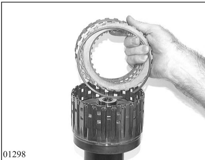
Insert complete disc set E. Starting with the spring disc 71.140, then alternately insert outer disc 71.150 and lining disc 71.160.
