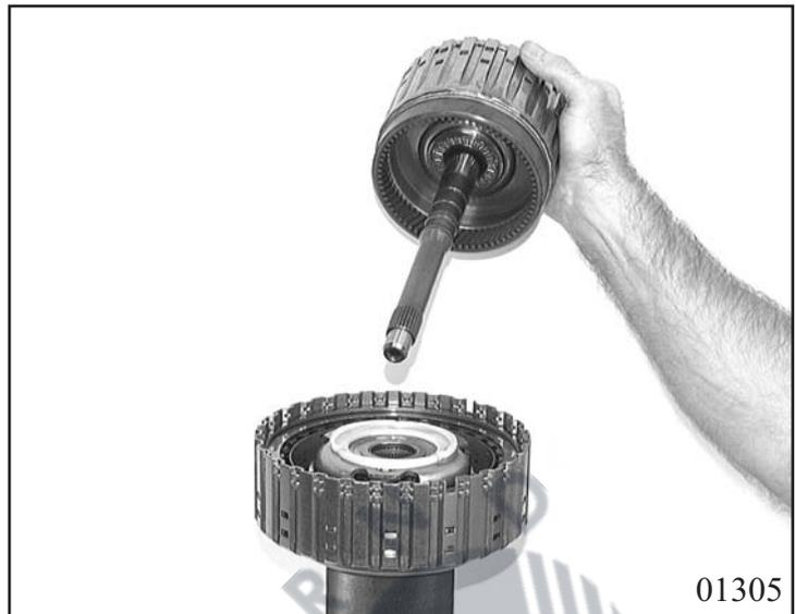
Align the discs of clutches A and E and
