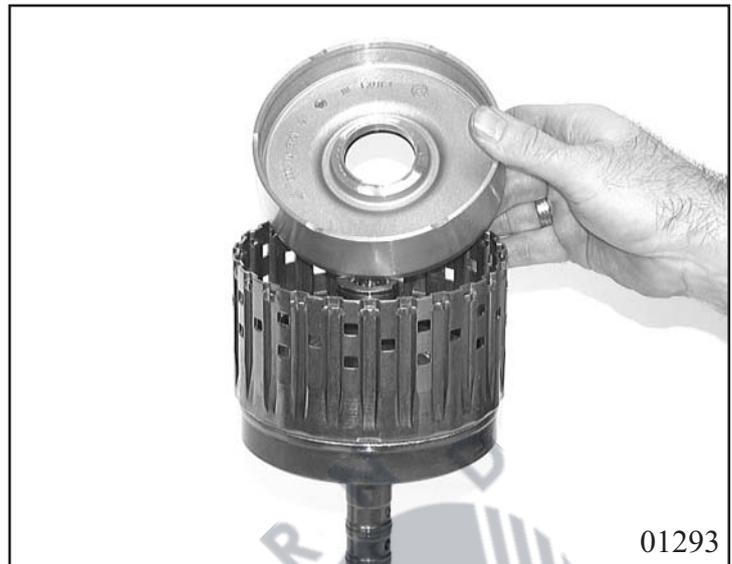
Pull on new round sealing ring 71.090 onto baffle 71.080. Insert cup spring 71.060 into cylinder E with protrusion downwards and press in baffle.
