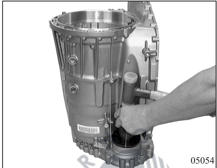
Take up gearbox housing in assembly bracket 5t66 000 128 and attach to assembly carriage or workbench holder 5x46 000 763.
