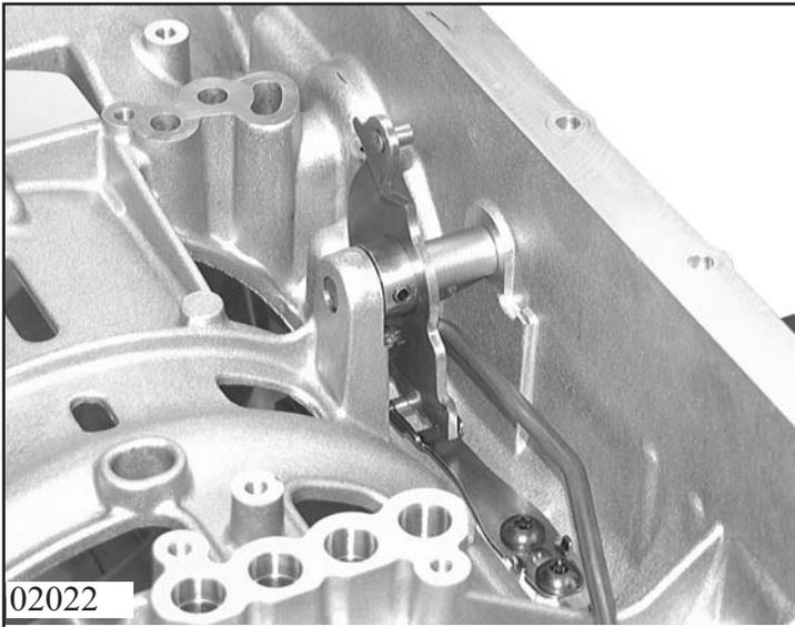
Align interlock spring with centring device Align 5x46 002 292 and tighten the interlock spring in this position. Tighten the screw on the side first.
