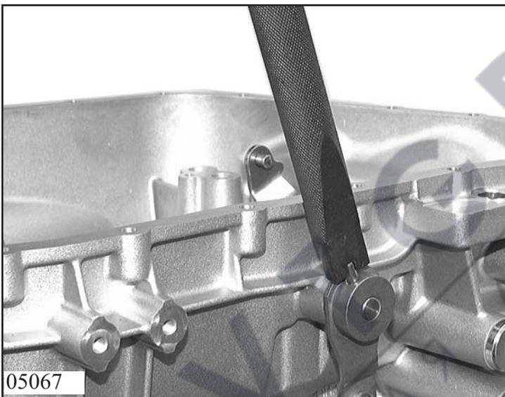
Attach shift lever to selection shaft and fix new clamping sleeve 06.160 in position shown with impact mandrel 5x46 000 291
