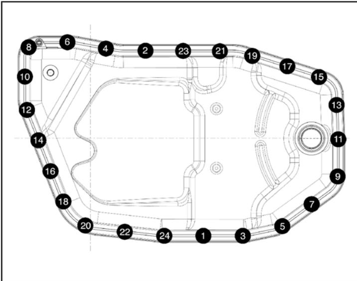
Tighten the oil pan torques according to the numbering:
