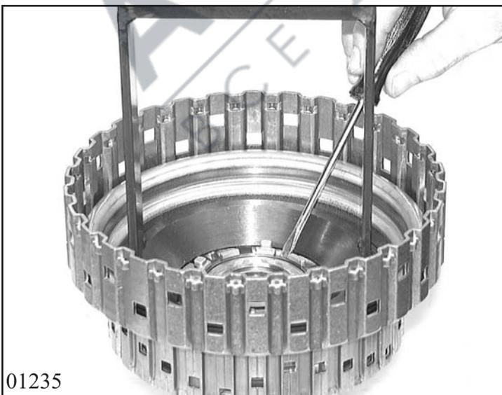
Press down diaphragm spring B with assembly bracket 5x46 002 566 under the mandrel press, remove snap ring. Remove disc and cup spring.
