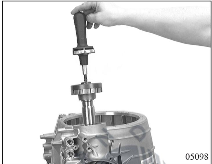
Insert snap ring 35.070 with pliers. Fit sleeve 5x46 909 344 onto pinion shaft. Push SSR 35.076 over sleeve and knock into converter bell with knock-in mandrel 5x46 909 269 up to stop.
