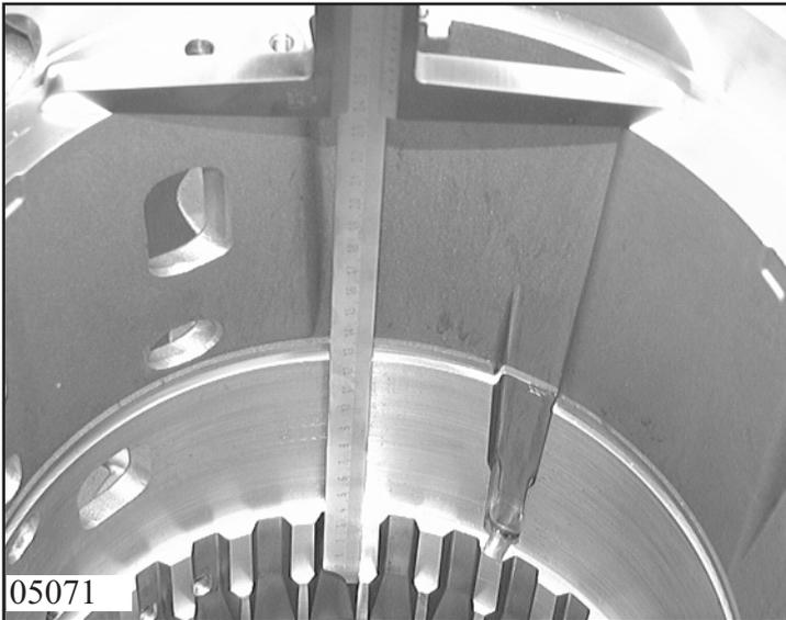
Measure brake D installation space  $E_D$  with depth gauge.
