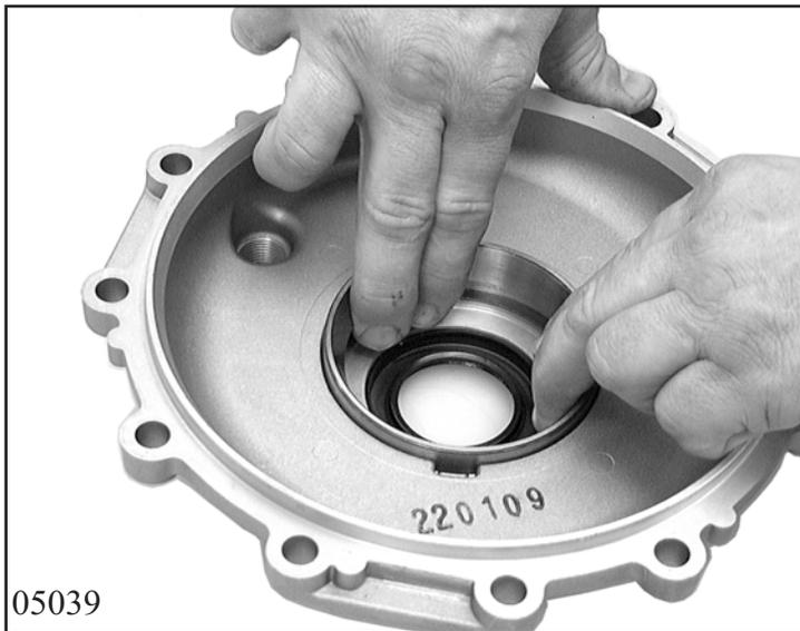
Remove round sealing ring. Remove bearing shell and setting shim, usually by hand, if necessary using tool 5x46 022 002 combined with tool 5x46 021 008. Pry off shaft sealing ring with suitable tools.
