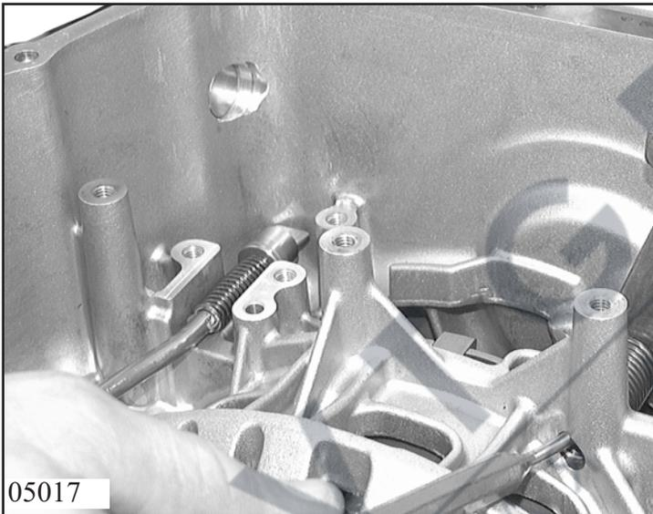
Drive out clamping sleeve from shift lever and remove shift lever.
