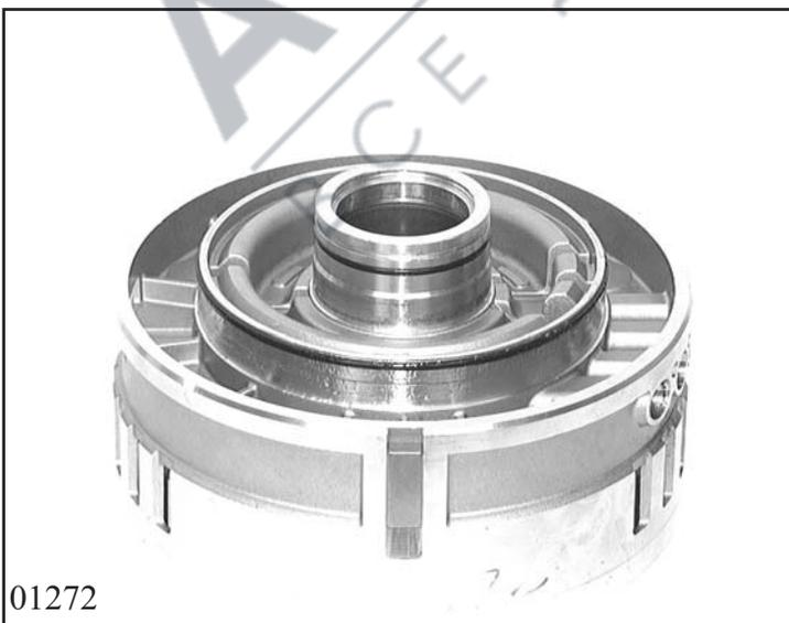
Knock in 2 adjusting springs 75.010/140 centrally at cylinder CD 75.010 with plastic hammer.
