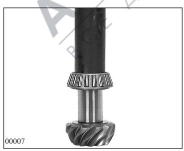
Fit shim washer 35.050 on pinion shaft 35.010/130 {part of complete bevel gear (paired)}.
