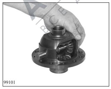
Turn planet gears through 90° about the differential axis and remove through inspection window together with thrust washer.
