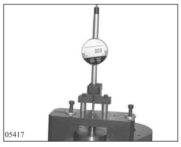
Position measuring bridge 5p01 000 357 with clock gauge above pressure pad. Set gauge to "0".
