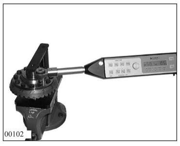
Clamp fitting 5x46 002 167 in vice, place differential in fitting, and screw crown gear to differential cage 35.010/110 with 12 new screws 35.010/140 using torque wrench with yield strength control, Quantec EMS ISI No. 7086.
